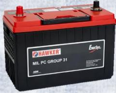
Generally, when fast (a.k.a., recovery) charging a single 12-volt **Hawker®**, an ideal **charger should have an output voltage between 14.4 to 15.0 VDC**. The optimal constant voltage is 14.7 VDC when the battery's temperature is at 77° F. Under normal conditions (when the **battery's** temperature is at or above 68° F), *it's not recommended to use a charger whose output voltage is less than 14.15 VDC or exceeds 15.0 VDC.*
