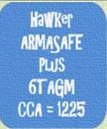
**Cold Cranking Amps (CCA)** is a standard battery industry rating referring to the amount of cranking power that a fully-charged battery has for engine start when temperatures are very cold. Specifically, it's the amount of amps that a nominal 12-volt battery can deliver at 0°F (-18°C) for 30 seconds while still maintaining at least 7.2 volts (that's 1.2 volts per cell). For example, the Hawker® ARMASAFE™ Plus battery has a CCA rating of **1225 amps**.
